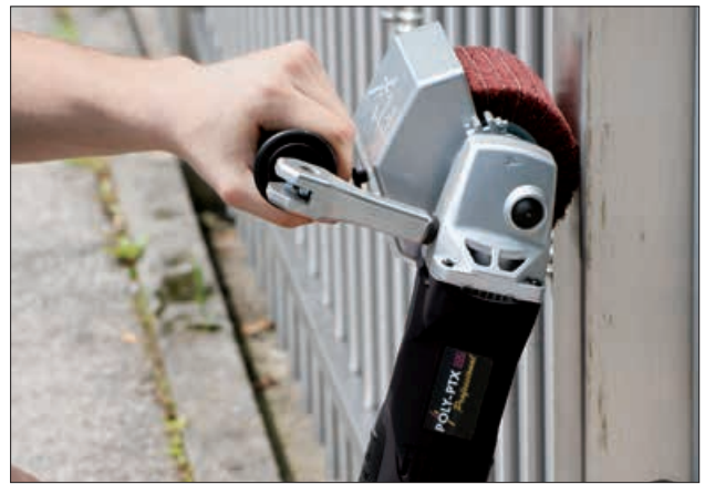
Satin finishing using interleaf fleece wheel.
