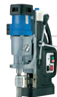
MAB 825, MAB 825 V & MAB 845, MAB 845 V p. 48-49 Capacity: \varnothing 4-1/16" cutter; \varnothing 1-1/4" twist drill; \varnothing 1-1/8" tapping Auto feed (MAB 825 V), Swivel base (MAB 845 & MAB 845 V), Reversible, 4-gear motor
