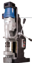
MAB 1300 & MAB 1300 V p. 50-52 Capacity: \varnothing 6" cutter \varnothing 1-3/4" twist drill \varnothing 1-5/8" tapping Reversible, 4-gear motor Auto-feed and reverse (MAB 1300 V) The ultimate in power
