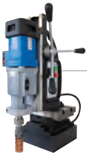
MAB 825 KTS p. 46-47 Capacity: \varnothing 3-1/8" cutter; \varnothing 1-1/4" twist drill; \varnothing 1-3/16" tapping; \varnothing 5" milling at 1" depth Portable magnetic mill drill for boring, slotting, etc. Reversible, 4-gear motor
