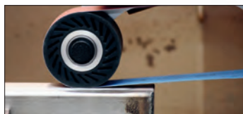
3 The drive roller with the rubber rings ensures that the grinding belts will not slip.
