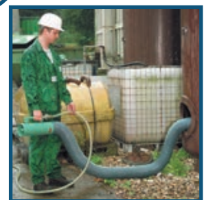
8 1620 0010 Pneumatic Air Mover, 7" dia. 2366 cfm output @ 90 psi
